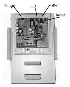
Figure 1 PIR with cover removed
